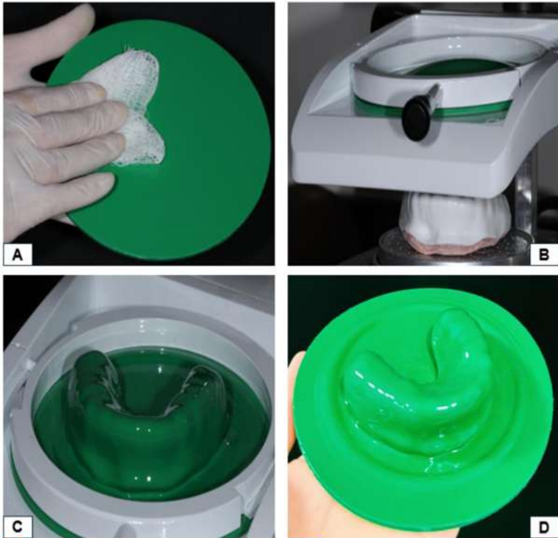
A: Cleaning the second plate with 70% alcohol; B: Second plate being inserted into the thermoplasticizer; C: Second thermoplasticized plate; D: Second thermoplasticized plate - pre-finishing.
