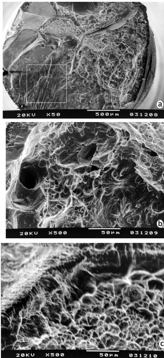
**Figure 4.** SEM images of sample F (a) 50x and (b) 500x regarding the circle, showing the dimples presence and (c) 500x regarding the square, showing the cleavage presence, after mechanical cycling test.
